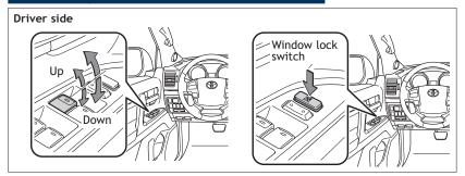
**Automatic operation** Push the switch completely down or pull it completely up and release to fully open or close. To stop window midway, lightly push the switch in the opposite direction.
